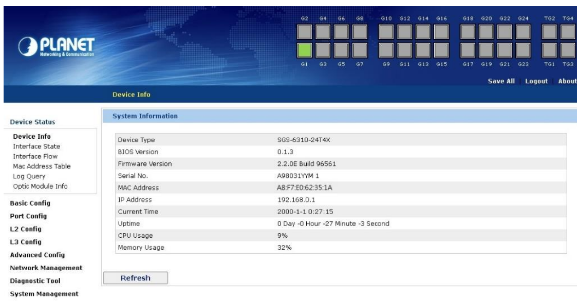
Figure 2-4-3: Web Main Screen of Managed Switch
